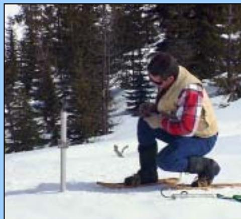
Reclamation and the USDA Natural Resource Conservation Service will continue to construct and manage SnoTel sites across the West that measure and record real-time snow pack data used to develop runoff forecasts for entire watersheds. Such partnerships would be expanded to include watersheds that are suffering shortages of both water and adequate data used to predict and forecast water supply.
